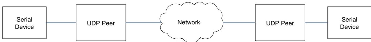
Figure 28-1 : Serial Data Point to Point
