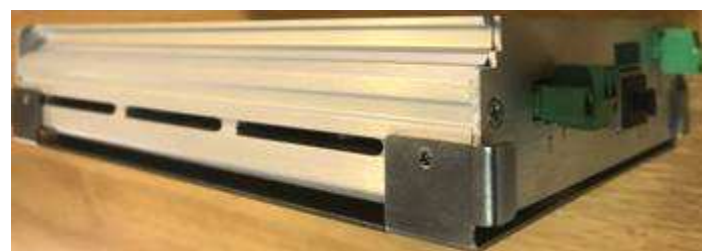
Rear view inc. Bracket (showing power connectors and 1x non-PoE Ethernet port)
