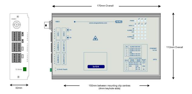
The **AMG5915** is a standalone one channel video transmit unit designed to transmit 1 video signal and transmit and receive 3 data signals plus 8 uni-directional alarms and also provides full duplex 100Base-T Ethernet connectivity over one Singlemode optical fibre.
