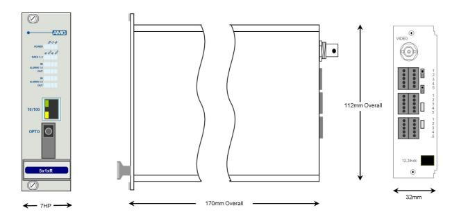
The **AMG5914R** is a rackmount one channel video receive unit designed to receive 1 video signal and transmit and receive 2 data signals plus 8 bi-directional alarms and also provides full duplex 100Base-T Ethernet connectivity over one Singlemode optical fibre.
