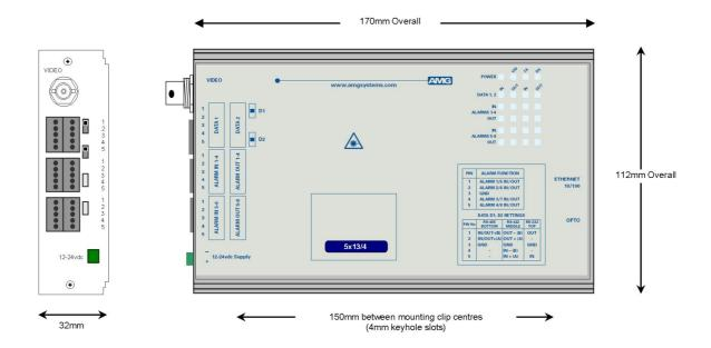
The **AMG5914** is a standalone one channel video receive unit designed to receive 1 video signal and transmit and receive 2 data signals plus 8 bi-directional alarms and also provides full duplex 100Base-T Ethernet connectivity over one Singlemode optical fibre.
