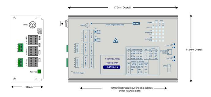
The **AMG5913-2A9** is a standalone one channel video transmit unit designed to transmit 1 video signal and transmit and receive 2 data signals, 2 audio channels plus 8 bi-directional alarms and also provides full duplex 100Base-T Ethernet connectivity over one Singlemode optical fibre.
