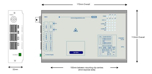
The **AMG5913** is a standalone one channel video transmit unit designed to transmit 1 video signal and transmit and receive 2 data signals plus 8 bi-directional alarms and also provides full duplex 100Base–T Ethernet connectivity over one Singlemode optical fibre.
