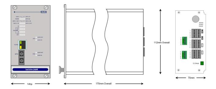
The **AMG5904-2A9R** is a rackmount data/audio receive unit designed to transmit and receive 2 data signals, 2 audio channels plus 8 bi-directional alarms and also provides full duplex 100Base-T Ethernet connectivity over a Singlemode optical fibre.
