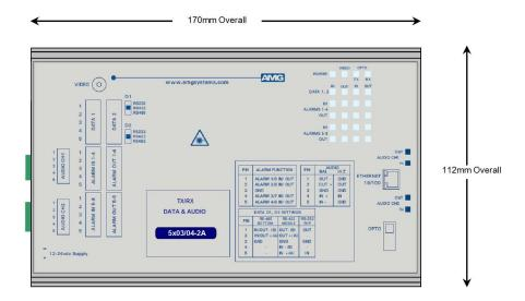
The **AMG5904-2A9** is a standalone data/audio receive unit designed to transmit and receive 2 data signals, 2 audio channels plus 8 bi-directional alarms and also provides full duplex 100Base-T Ethernet connectivity over a Singlemode optical fibre.
