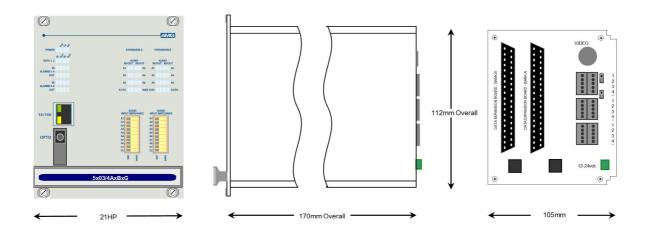
The **AMG5903A966B9G** is a rackmount data transmit unit designed to transmit and receive 2 data channels, 14 audio channels, 2 Echelon FTT-10A data channels and 8 bi-directional alarms over one Singlemode optical fibre. It also provides full duplex 100BASE-TX Ethernet connectivity.
