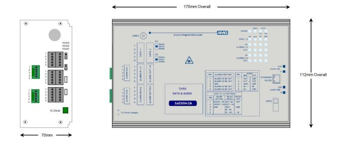
The **AMG5903-2A9** is a standalone data/audio transmit unit designed to transmit and receive 2 data signals, 2 audio channels plus 8 bi-directional alarms and also provides full duplex 100Base-T Ethernet connectivity over a Singlemode optical fibre.
