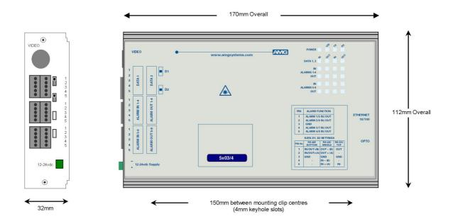
The **AMG5903** is a standalone data transmit unit designed to transmit and receive 2 data signals plus 8 bi-directional alarms and also provides full duplex 100Base-T Ethernet connectivity over one Singlemode optical fibre.
