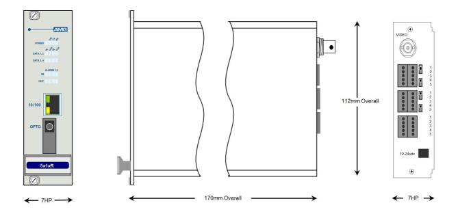
The **AMG5818R** is a rackmount one channel video receive unit designed to receive 1 video signal and transmit and receive 4 data signals plus 4 bi-directional alarms and also provides full duplex 100Base-T Ethernet connectivity over one Multimode optical fibre.
