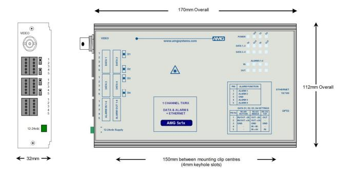
The **AMG5818** is a standalone one channel video receive unit designed to receive 1 video signal and transmit and receive 4 data signals plus 4 bi-directional alarms and also provides full duplex 100Base-T Ethernet connectivity over one Multimode optical fibre.
