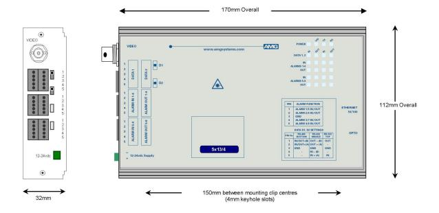
The **AMG5814-DF** is a standalone one channel video receive unit designed to receive 1 video signal and transmit and receive 2 data signals plus 8 bi-directional alarms and also provides full duplex 100Base-T Ethernet connectivity over two Multimode optical fibres.
