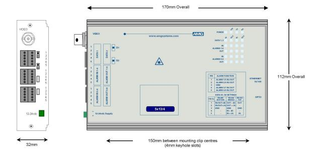
The **AMG5813-DF** is a standalone one channel video transmit unit designed to transmit 1 video signal and transmit and receive 2 data signals plus 8 bi-directional alarms and also provides full duplex 100Base-T Ethernet connectivity over two Multimode optical fibres.
