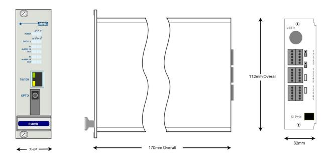
The **AMG5804R** is a rackmount receive unit designed to transmit and receive 2 data signals plus 8 bidirectional alarms and also provides full duplex 100Base-T Ethernet connectivity over one Multimode optical fibre.
