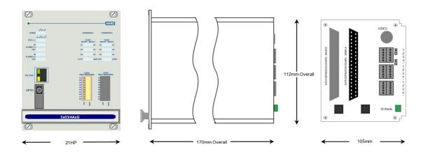
The **AMG5804A966G** is a rackmount data receive unit designed to transmit and receive 2 data channels, 6 audio channels, 2 Echelon FTT-10A data channels and 8 bi-directional alarms over one Multimode optical fibre. It also provides full duplex 100Base-T Ethernet connectivity.
