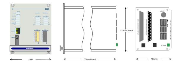
The **AMG5803A966G** is a rackmount data transmit unit designed to transmit and receive 2 data channels, 6 audio channels, 2 Echelon FTT-10A data channels and 8 bi-directional alarms over one Multimode optical fibre. It also provides full duplex 100Base-T Ethernet connectivity.
