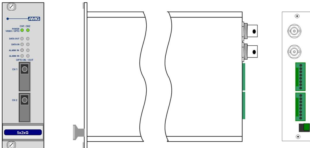
The **AMG5626G** is a **DUAL** rackmount system which provides two independent channels, each designed to receive 1 video signal plus 2 uni-directional alarms and transmit and receive 1 data signal over a single Multimode optical fibre.
