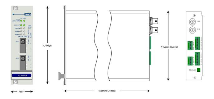
The **AMG5626A1R** is a **DUAL** rackmount system which provides two independent channels, each designed to receive 1 video signals plus 2 Uni-directional alarms and transmit and receive 2 data signals over one Multimode optical fibre.
