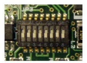
The switch functions are as follows: Default (RS-485) settings are shown in the last column.
