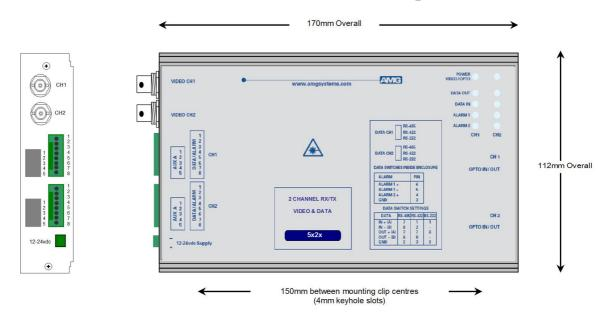
The **AMG5626** is a **DUAL** standalone system which provides two independent channels, each designed to receive 1 video signal plus 2 uni-directional alarms and transmit and receive 1 data signal over one Multimode optical fibre.
