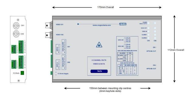
The **AMG5625A1** is a **DUAL** rackmount system which provides two independent channels, each designed to transmit 1 video signals plus 2 Uni-directional alarms and transmit and receive 2 data signals over one Multimode optical fibre.
