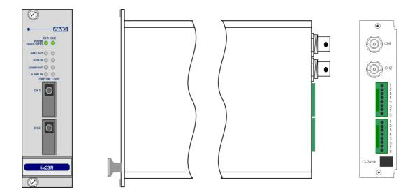
The **AMG5623R** is a **DUAL** rackmount system which provides two independent channels, each designed to transmit one video signal and transmit and receive one bi-directional alarm plus one data signal over one Multimode optical fibre.
