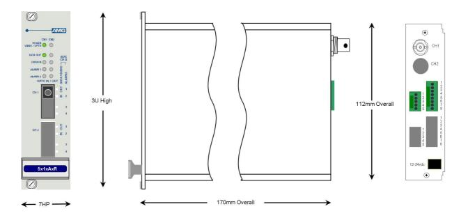
The **AMG5616A9R** is a rackmount one channel video receive unit designed to receive 1 video signal plus 2 Uni-directional alarms, and transmit & receive 1 data signal plus 1 Bi-directional audio channel over a single Multimode optical fibre.
