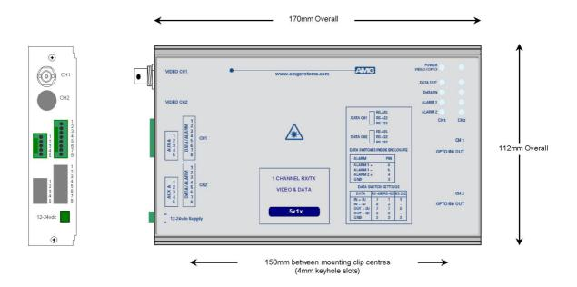
The **AMG5616A9** is a standalone one channel video receive unit designed to receive 1 video signal plus 2 Uni-directional alarms, and transmit & receive 1 data signal plus 1 Bi-directional audio channel over a single Multimode optical fibre.
