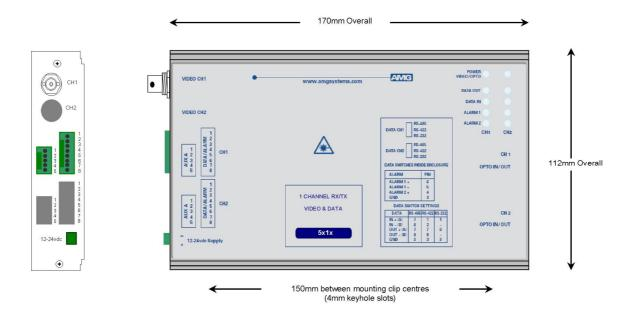
The **AMG5616A1** is a standalone one channel video receive unit designed to receive 1 video signal plus 2 Uni-directional alarms, and transmit & receive 2 data signals over a single Multimode optical fibre.
