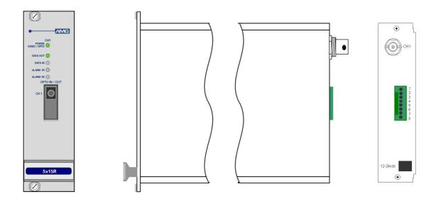
The **AMG5615R** is a rackmount one channel video transmit unit designed to transmit 1 video signal plus 2 Uni-directional alarms and transmit and receive 1 data signal over one Multimode optical fibre.
