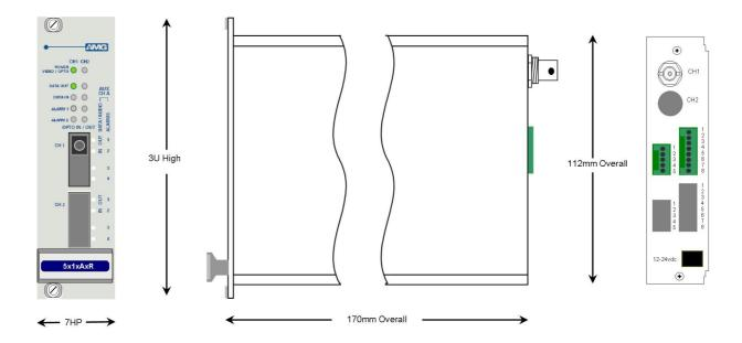
The **AMG5615A9R** is a rackmount one channel video transmit unit designed to transmit 1 video signal plus 2 Uni-directional alarms, and transmit & receive 1 data signal plus 1 Bi-directional audio channel over a single Multimode optical fibre.
