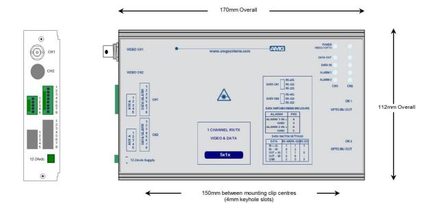
The **AMG5615A9** is a standalone one channel video transmit unit designed to transmit 1 video signal plus 2 Uni-directional alarms, and transmit & receive 1 data signal plus 1 Bi-directional audio channel over a single Multimode optical fibre.
