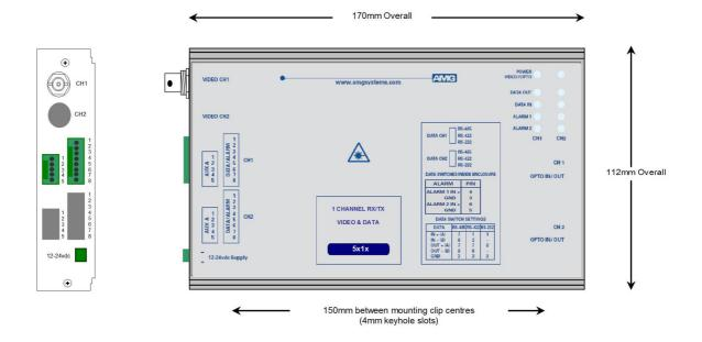
The **AMG5615A5** is a standalone one channel video transmit unit designed to transmit 1 video signal plus 2 Uni-directional alarms, and transmit & receive 1 data signal plus 1 Bi-directional alarm over a single Multimode optical fibre.
