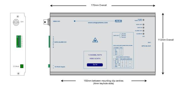
The **AMG5614** is a standalone system designed to receive one video signal and transmit and receive one bi-directional alarm plus one data signal over a Multimode optical fibre.
