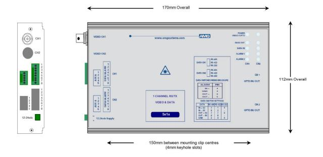
The **AMG5614A3** is a standalone one channel video receive unit designed to receive 1 video signal and transmit & receive 1 RS485/RS232/RS422 data signal and 1 20mA current loop data signal plus 1 Bi-directional alarm over a single Multimode optical fibre.
