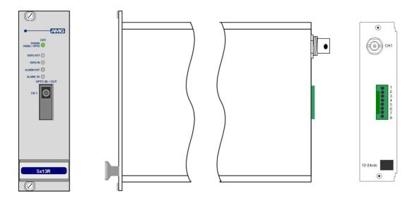
The **AMG5613R** is a rackmount one channel video transmit unit designed to transmit 1 video signal and transmit and receive 1 data signal plus 1 bi-directional alarm over one Multimode optical fibre.
