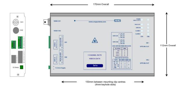
The **AMG5613A3** is a standalone one channel video transmit unit designed to transmit 1 video signal and transmit & receive 1 RS485/RS232/RS422 data signal and 1 20mA current loop data signal plus 1 Bi-directional alarm over a single Multimode optical fibre.
