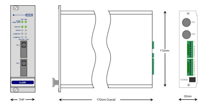
The **AMG5426R** is a **DUAL** rackmount data receive unit which provides two independent channels, each designed to receive 2 uni-directional alarms and transmit and receive 1 data signal over one Multimode optical fibre.
