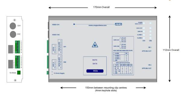
The **AMG5426** is a **DUAL** standalone system which provides two independent channels, each designed to receive 2 uni-directional alarms and transmit and receive 1 data signal over one Multimode optical fibre.
