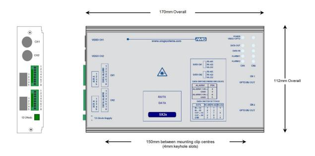
The **AMG5425** is a **DUAL** standalone system which provides two independent channels, each designed to transmit 2 uni-directional alarms and transmit and receive 1 data signal over one Multimode optical fibre.
