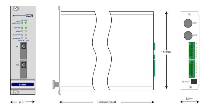
The **AMG5424R** is a **DUAL** rackmount data receive unit which provides two independent channels, each designed to transmit and receive 1 bi-directional alarm and transmit and receive 1 data signal over one Multimode optical fibre.
