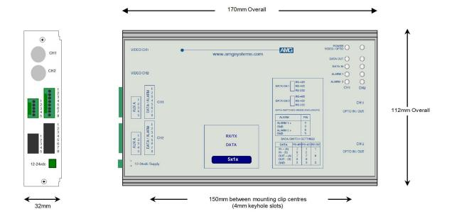
The **AMG5413A9** is a standalone transmit unit designed to transmit & receive one Bi-directional alarm, one Bi-directional audio channel and one Bi-directional data signal over a Multimode optical fibre.
