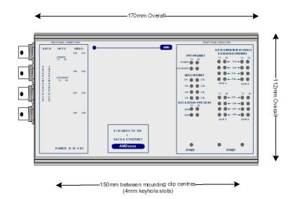
The **AMG4687BE** is a standalone eight channel video transmit unit designed to transmit 8 video signals and transmit and receive up to 9 data or audio signals plus full duplex 100BaseT Ethernet connectivity over two Multimode fibres. The 9 data/audio channel interfaces, whether RS232, RS422, RS485, 20mA, TTL, Contact Closure, Lonworks or Audio, are defined at manufacture by the addition of daughter boards fitted onto the Data Expansion Board B.
