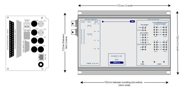
The **AMG4627B** is a standalone two channel video transmit unit designed to transmit 2 video signals and transmit and receive up to 9 data or audio signals over two Multimode fibres. The 9 data/audio channel interfaces, whether RS232, RS422, RS485, 20mA, TTL, Contact Closure, Lonworks or Audio, are defined at manufacture by the addition of daughter boards fitted onto the Data Expansion Board B.
