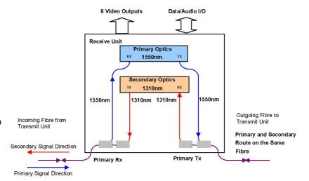
As each unit regenerates the optical signal, the optical dynamic range between each optically connected node is 17dB.
