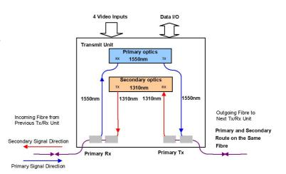
The AMG3747R-DR-SF receives and drops off data signals transmitted from an AMG3788N-DR-SF or AMG3788RN-DR-SF receiver. It then inserts video and data signals onto the outgoing optical signal.
