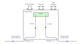
The **AMG3747BE** receives and drops off data & Ethernet signals transmitted from an **AMG3788E** receiver. It then inserts video, data and Ethernet signals onto the outgoing optical signal.
