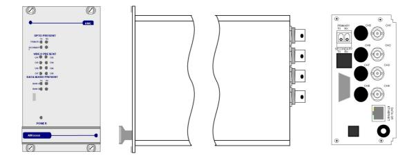
The **AMG3741EG-DR-SF** is a rackmount four channel video insert unit designed to transmit 4 video signals onto a singlemode optical fibre ring with Dual Redundant operation. It also provides full duplex 100BaseT Ethernet connectivity around the ring.
