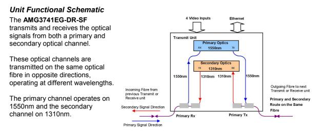
The AMG3741EG-DR-SF receives and drops off Ethernet signals transmitted from an AMG3782EGN-DR-SF receiver, it then inserts video and Ethernet signals onto the outgoing optical signal.
