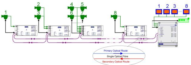
If a fibre link is broken, operation of the ring continues by making use of the secondary optical fibre route as below:
