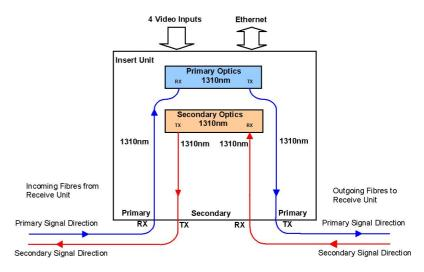
As each unit regenerates the optical signal, the optical dynamic range between each optically connected node is 17dB.
