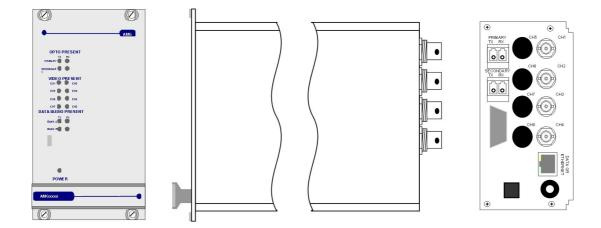
The **AMG3741EG-DR** is a rackmount four channel video insert unit designed to transmit 4 video signals onto a dual singlemode optical fibre ring with Dual Redundant operation. It also provides full duplex 100BaseT Ethernet connectivity around the ring.
