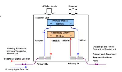
The AMG3741E-DR-SF receives and drops off Ethernet signals transmitted from an AMG3782ERN-DR-SF receiver, it then inserts video and Ethernet signals onto the outgoing optical signal.
