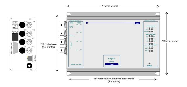
The **AMG3741E-DR-SF** is a standalone four channel video insert unit designed to transmit 4 video signals onto a singlemode optical fibre ring with Dual Redundant operation. It also provides full duplex 100BaseT Ethernet connectivity around the ring.
