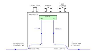
The **AMG3727BE** receives and drops off data & Ethernet signals transmitted from an **AMG3788E** receiver. It then inserts video, data and Ethernet signals onto the outgoing optical signal.
