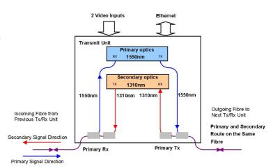
The AMG3721E-DR-SF receives and drops off Ethernet signals transmitted from an AMG3782E-DR-SF receiver. It then inserts video and Ethernet signals onto the outgoing optical signal.
