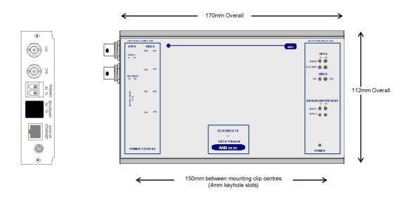
The **AMG3721E-DR-SF** is a standalone single channel video insert unit designed to transmit two video signals onto a singlemode optical fibre ring with Dual Redundant operation. It also provides full duplex 100BaseT Ethernet connectivity around the ring.
